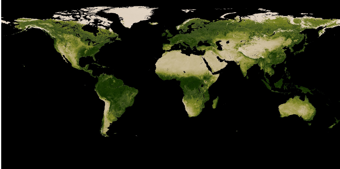
Fig 1: Monitoring Vegetation through MODIS NDVI Data at 0.25 degrees resolution. (Imagery produced by the NASA Earth Observations team using data provided by the MODIS Land Science Team.)
